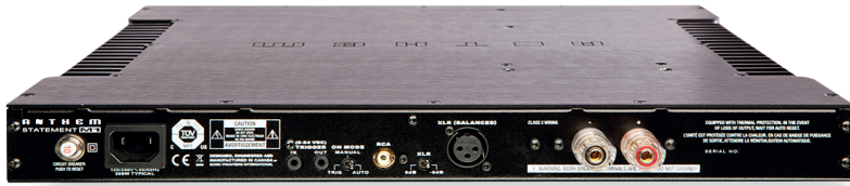
ABOVE: In keeping with its 'custom installation' brief, the M1 may be switched out of standby via trigger, via signal auto-sensing or manually. The single-ended (RCA) and balanced (XLR) inputs are also switched but the 4mm speaker outlets are fixed
