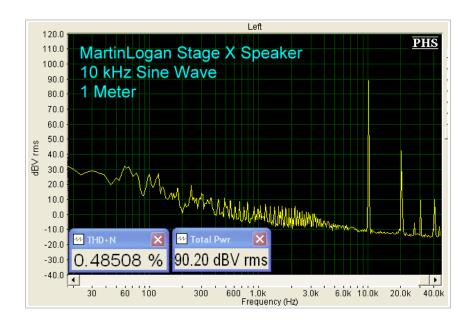
Here is the room frequency response, at 1 meter, on-axis. You can see the dip in the midrange that I heard. Again, this can be managed, if you wish, with your processor's room correction feature. Response falls off rapidly below  $60\,\mathrm{Hz}$
