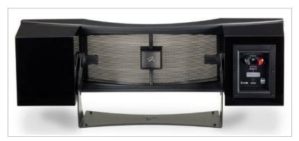
The speaker binding posts are five way. A small jack is at the bottom for connecting a wall-wart cable that supplies bias voltage to the thin membrane between the stators.
